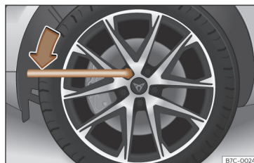
Fig. 41 Wheel change: loosen the wheel nuts.
