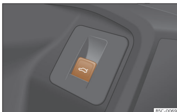
Fig. 88 On the driver's door: button to open and close the rear lid.
