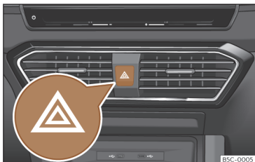
Fig. 97 Dash panel: hazard warning lights switch
