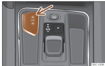
Fig. 75 Centre console: vehicle key socket.
