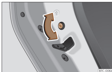
Fig. 85 Childproof lock on the left hand side door.
