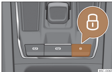
Fig. 80 In the centre console: central locking switch
