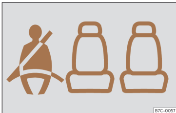
Fig. 9 Instrument panel: left rear seat occupied and corresponding seat belt fastened display.
