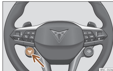
Fig. 159 Multifunction steering wheel: button to change the driving profile.
