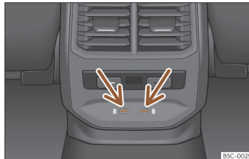
Fig. 153 Rear part of the centre console: USB connectors with power outlet function.
