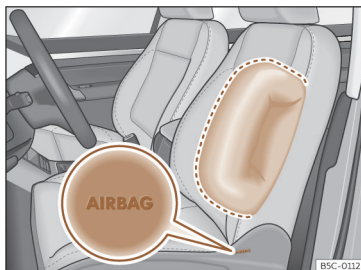
Fig. 25 Side airbag in driver's seat.
