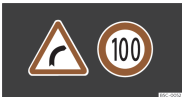
Fig. 58 On the instrument panel display: examples of recognised signals.
