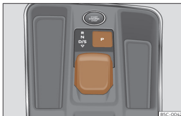
Fig. 157 In the centre console: selector lever.
